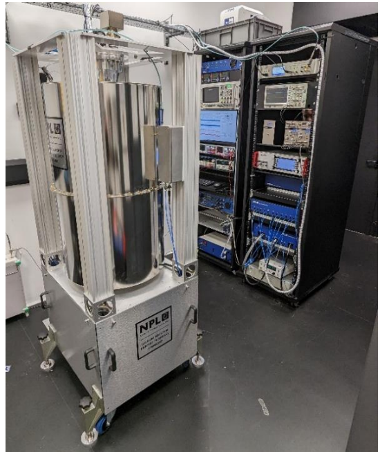
Fig. 1: One of the new generation of NPL Cs fountains, showing the physics package and two racks that make up the system.
